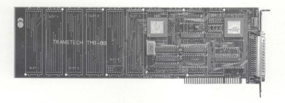
Introduction The TMB08 is a 10 TRAM motherboard for IBM PC XT and AT compatible machines. It incorporates a link crossbar switch (IMSC004) allowing user configuration of network topologies. Eight of the links connected to the C004 are hardwired to the D-type edge connector, allowing networks with external connections to be configured.
