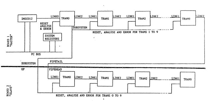
To allow the configuration of the slave board to be programmed from the master board the T212 link 1 ("config up") should be connected to the patch link 0 on the patch area, to allow it to be connected to the T212 on the master board via config down on the masterboard's edge connector.
