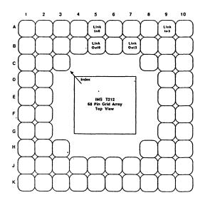
CONNECT PIN A5 TO B7 AND PIN B5 TO A9
