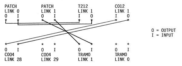
TRAMO should derive its system services control from the "UP" on the 37 way edge connector, hence jumper I should be in. TRAMs 1 to 9 and the T212 should also receive control from the "UP" so jumper 0 should be in too. The slave board is now configured and ready to be connected to the master board. The following connections need to be made between the two boards.
