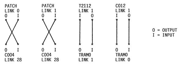
The other connections made on the patch area are Patch Link 0 and 1 connected to COO4 links 28 and 29, which provide two more (making 10 in all) link connections from the COO4 to the edge connector.
